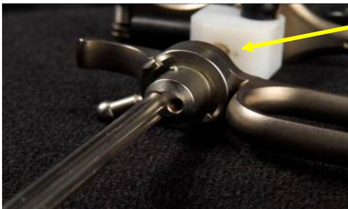
A hole within a Teflon block that is part of the resectoscope system's working element. While not obvious to the user, this hole comes into play when determining the reprocessing for this device.
